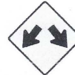
Lane Splits at Median
